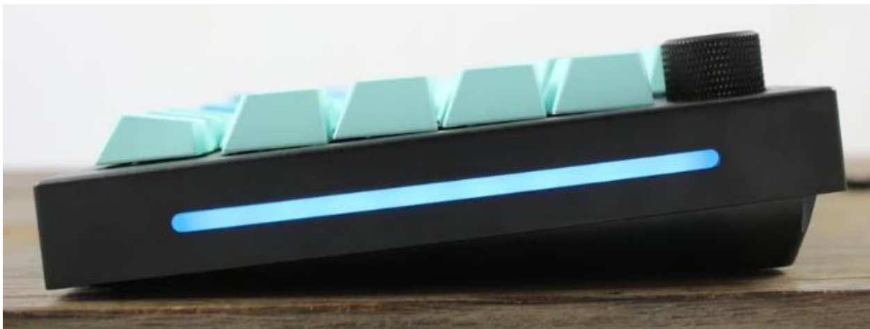
Figure 7.2: Plastic strip running along the side of the case allowing for RGB to shine through.
