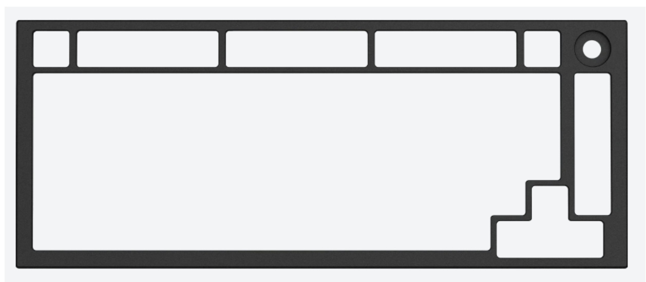
Figure 8: Aluminum Top Frame for the GMMK Pro
