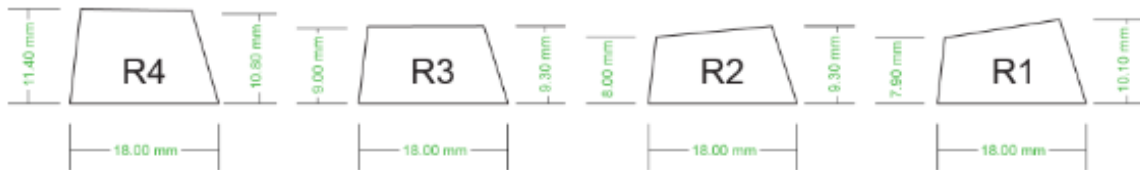
Figure 3.2: Measurements of the different rows of keycaps.
